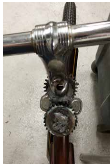
Above: Reassembled gears in the handlebar makes the bike steer in reverse.
